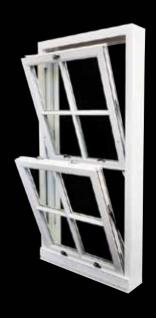
Our Traditional Style and Stormproof windows are constructed in standard section frames which are 95mm x 68mm with a 19mm ovlo, or heavy section frames which are 140mm x 68mm with a 19mm ovlo. Both Traditional and Stormproof style have a casement size of 68mm x 58mm.
